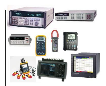
All kind of measuring indicator – DMM, Clamp, Calibrator, Recorder, Watt meters, Power Analyzer Handheld, Panel ndicator
